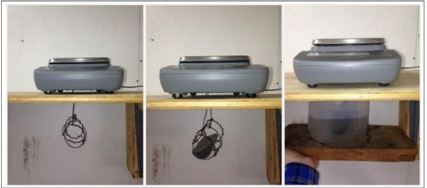
Figure 11-6: Bulk Density Measurement Equipment at Goldlund
