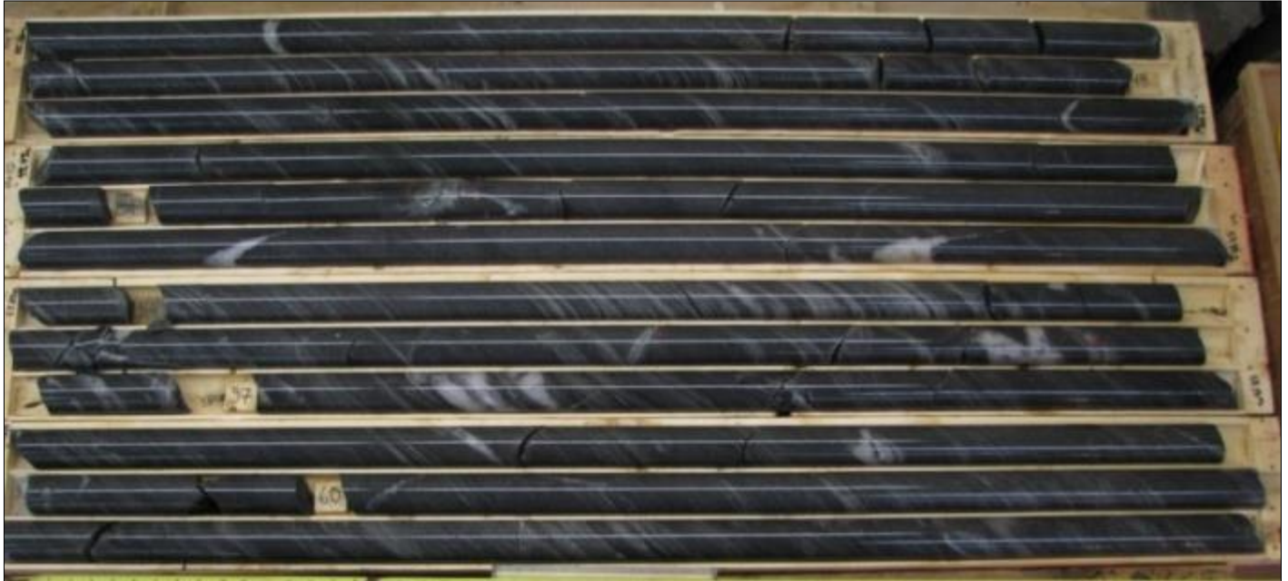
Figure 7-5: Dimond Drill Core Photograph showing BMS (top) and MSS (bottom)
